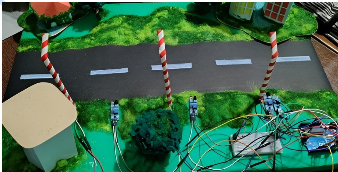
Figure 1: Smart Street Lighting System Model
